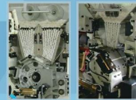
Double Plunger Hopper (Speed up to 180ppm) Single Plunger Hopper (Speed up to 150ppm)
